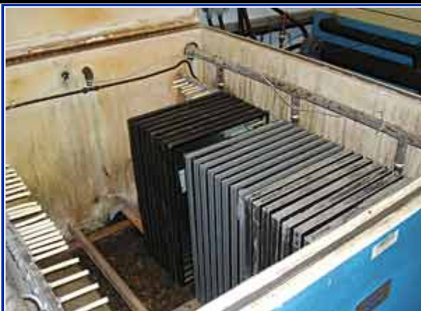
Insulating glass samples are subjected to high humidity and temperature tests.
